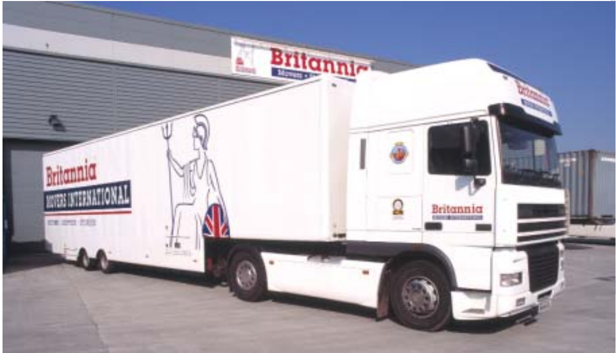
Articulated vehicle 18.5m long, 4m high, 2.5m wide capacity 110m 3 .
